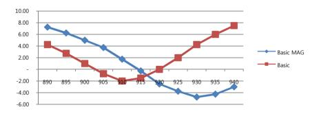
•BASIC MAG reads up to 4.0 meters on metal, 20% longer than BASIC. Its read performance varies upon tag location, orientation, direction, RF environments, etc.
